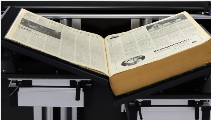
Scanning a book using the protective V cradle for fragile bound documents.
